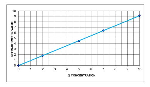
The data provided for the % concentration control is prepared according to the data obtained for the freshly prepared emulsion. As the utilization time of the emulsion and the undesired oil/contamination amount in the system increases, deviations from the data stated above should be taken into account.
